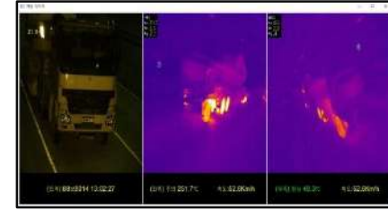
Over-heated vehicle detection System
