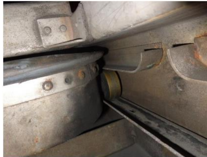
Figure 39 : rail galet non graissé
